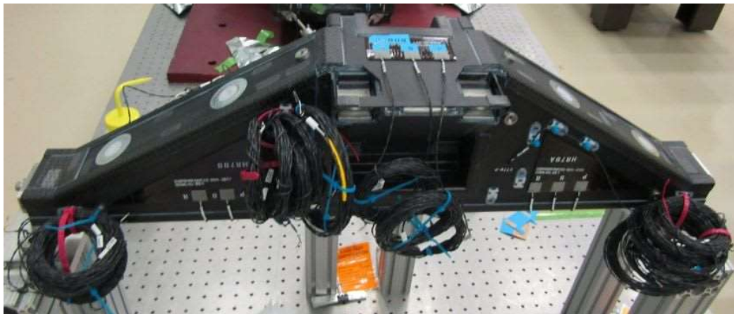
The Tertiary Optical Mirror Assembly (TOMA) completed with 3 powered mirrors installed to generate a low WFE collimated beam for the CGI and an actuated flat mirror to finely align the pupil position into the CGI.
