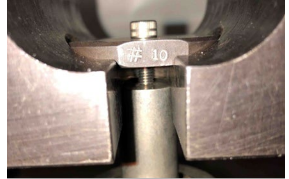
541 Short Tensile Setup
