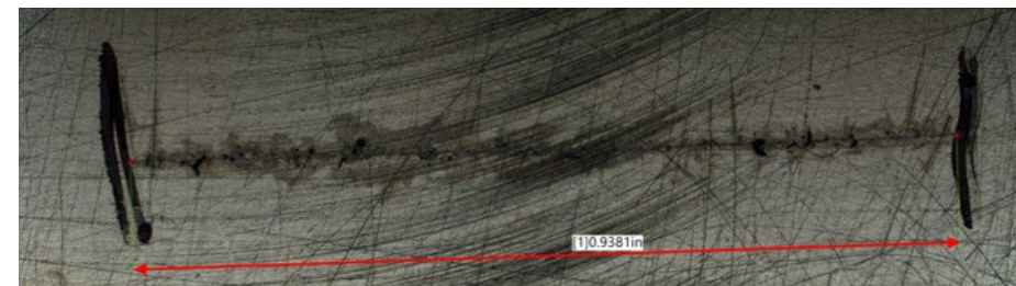
Pre-etch microscopy of an Inconel crack panel, after penetrant inspection
