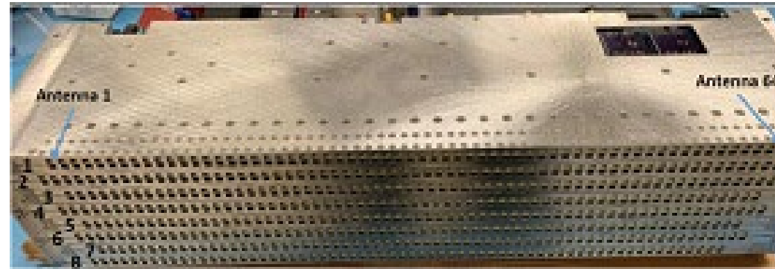
TRI and ISU's multi-static imaging array developed in the Phase II SBIR effort consisting of 8 linear arrays, each with 64 antennas (width is ~16").
