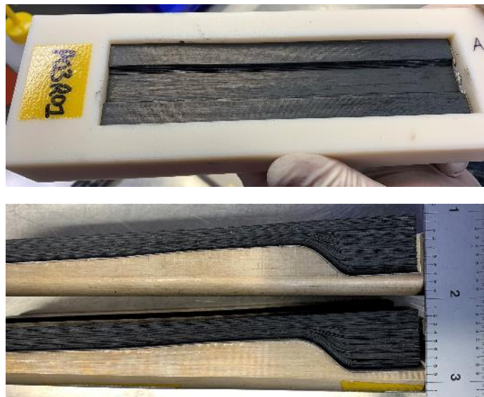
Figure 4.005 – Wet Layup Cavity
