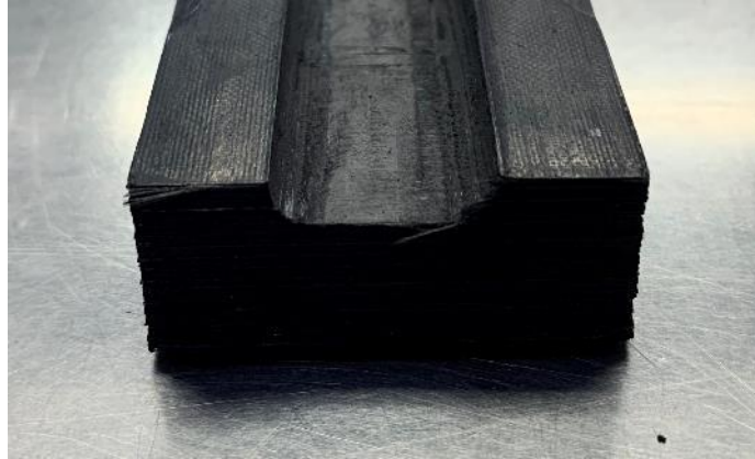
Figure 4.006 – Green State Machined Cavity
