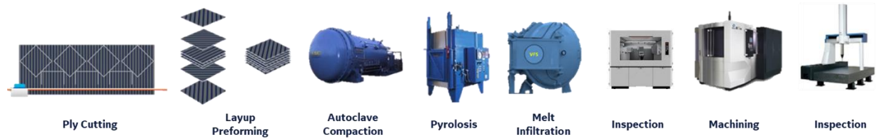
Figure 4.004 – MI SiC/SiC Composite Manufacturing Process
