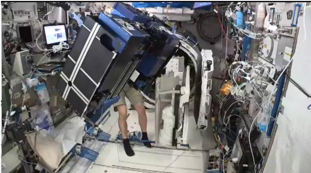
JAXA astronaut Soichi Noguchi installed the four MSCs, the MISSE Power and Data Box (MPD), and the MISSE Switch Box (MSB) on the MTT
