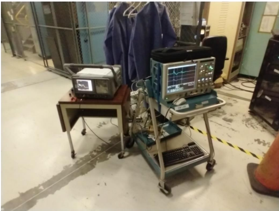
Spectrum Analyzer, Digital Oscilloscope Measuring EMI Lab F-65 Current Probe Output
