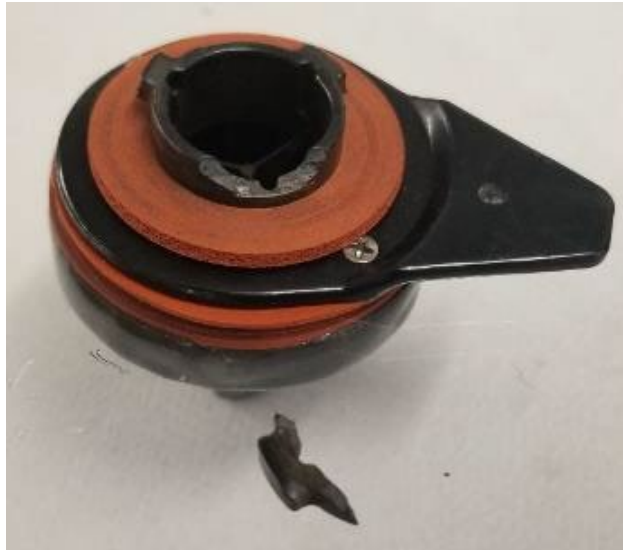
Figure 13: Broken bayonet fitting on one of the lids of a test chamber
