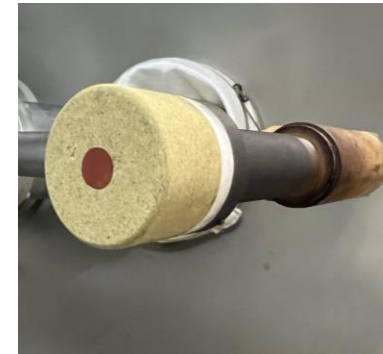
(a) Graphite sample embedded with TCs[2], (b) PICA assembly with RTV cylinder.
