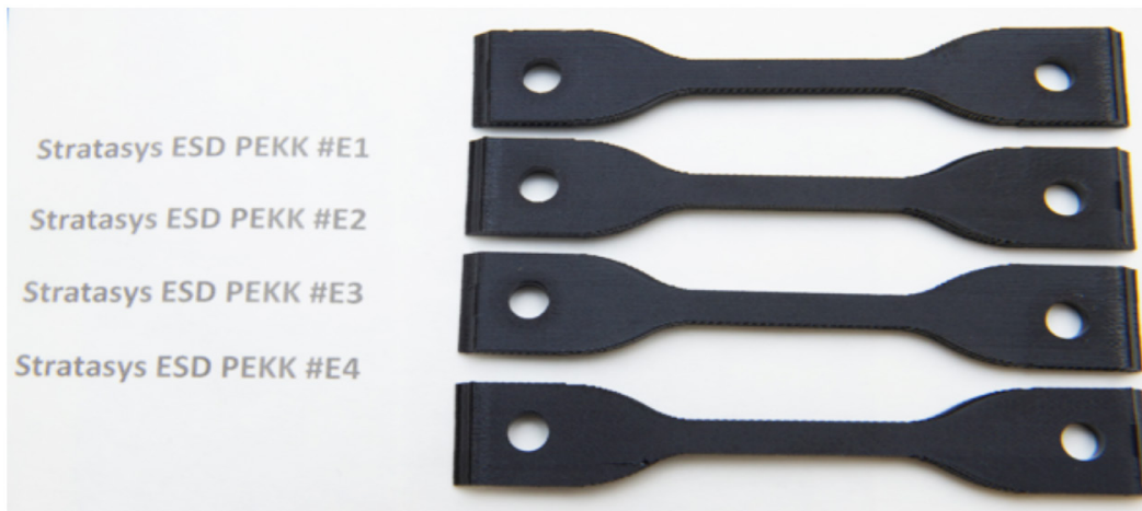
Figure 11. Stratasy ESD PEKK MISSE-9 post-flight samples (E1–E3) and one control sample (E4).
