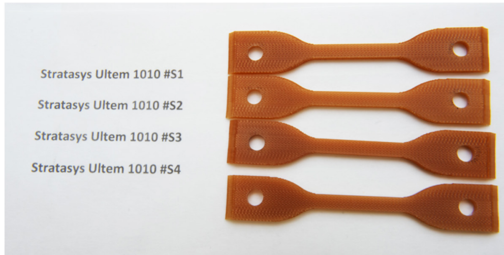
Figure 9. MISSE-9 Stratasys Ultem 1010 post-flight samples (S1–S3) and one control sample (S4).
