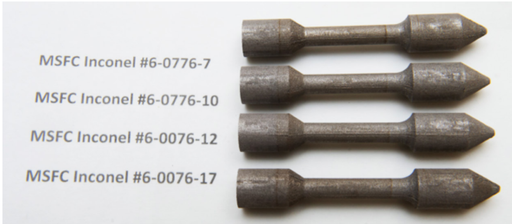
Figure 15. Inconel 718 MISSE-9 post-flight samples (top three) and one control sample (bottom).
