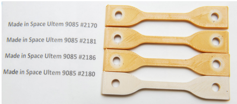
Figure 7. MISSE-9 MIS Ultem 9085 post-flight samples (2170, 2181, and 2186) and one control sample (2180).
