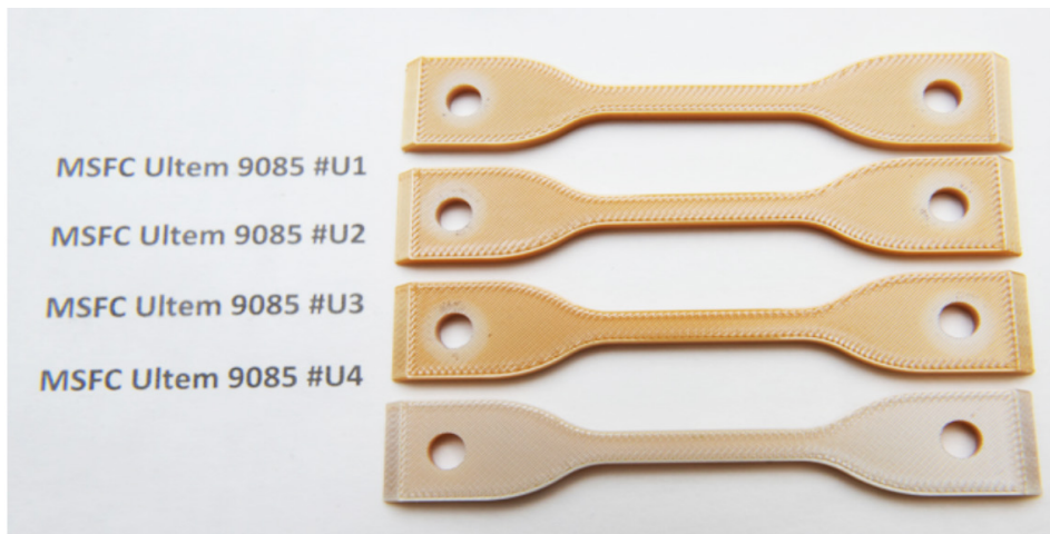
Figure 5. MISSE-9 MSFC Ultem 9085 three post-flight samples (U1-U3) and one control sample (U4).
