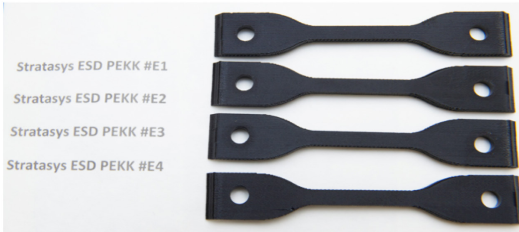
Figure 11. Stratasyes ESD PEKK MISSE-9 post-flight samples (E1–E3) and one control sample (E4).
