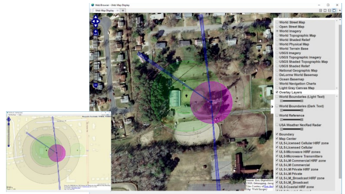
Fig. 5c: ULS transmitters HIRF zones example. Satellite view.
