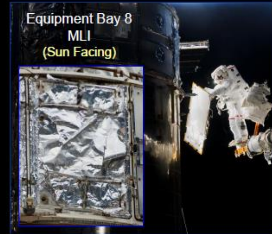
SM4 replacement of severely degraded Bay 8 MLI 19 years of space exposure
