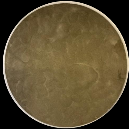
Sputter target made from simulant with chemistry closest to Mare Crisium
