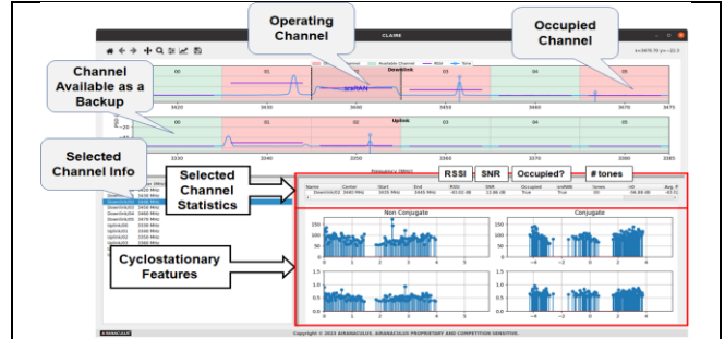
Figure 5. Wideband RF sensing User Interface - Signal processing flow consisting of spectrum segmentation, statistical signal processing, CSP and ML based detection and characterization, Channel Quality Estimation (CQE).
