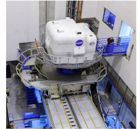
Vertical Motion Simulator (VMS) located at NASA Ames
