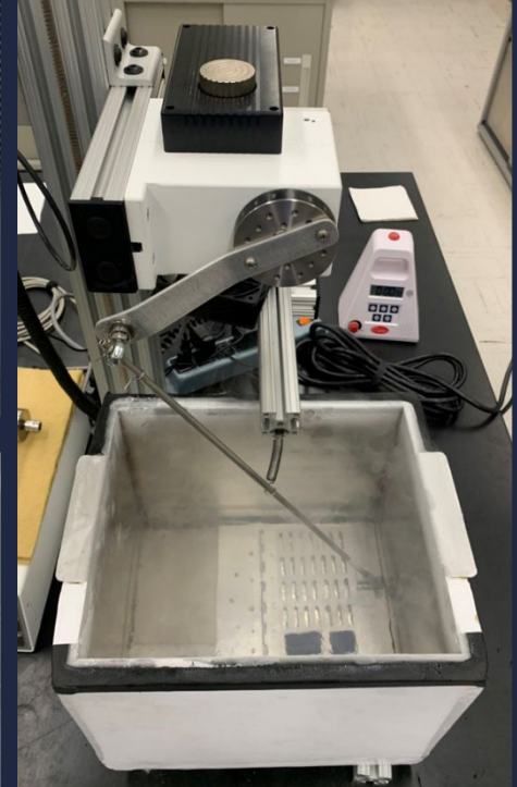
Instron strength test apparatus in LN2 chamber (upper left). Folding apparatus (lower left). LN2 bath with folding apparatus motor and interfaces (right). Image Credit: NASA
