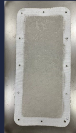
Fabric panel showing remaining lunar simulant after being removed from tumbler (left); Fabric panel showing strips cut for tensile testing (right) Image Credit: NASA
