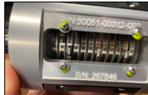
Slip ring must be rugged and provide reliable rotor-stator coupling
