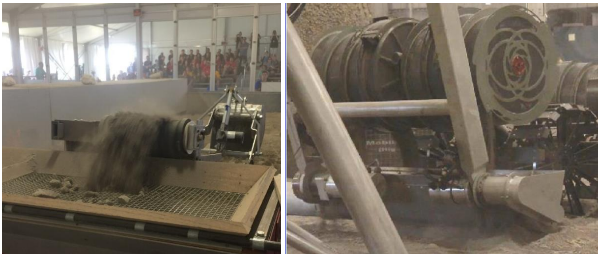
Figure 7. Left: At the 2016 NASA Robotic Mining Competition, a robot depositing regolith through a grizzly to remove rocks. Image: Metzger. Right: NASA’s RASSOR bucket drum excavator delivering regolith into a hopper containing an auger to push soil across openings that allow soil through while gravel is rejected out the end.
