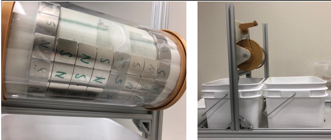
Figure 16. Magnetic Separator Experiment Apparatus.
