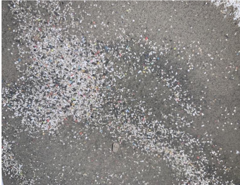
Figure 10. Plastic particles mixed in lunar soil simulant demonstrating easy segregation by particle size.
