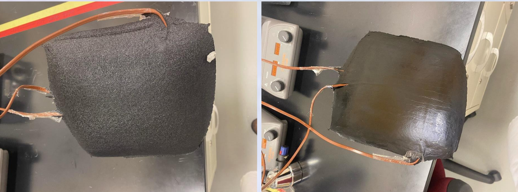
Green rubber insulation inoculated with 10 9 CFU/ml B. atrophaeus spores (top). Insulation panels post-cure (bottom).
