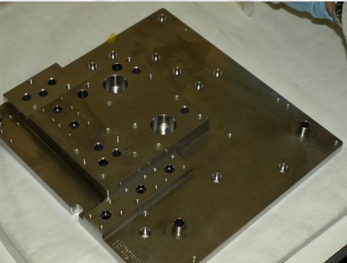
SERFE Backplate with Integrated Fluid Passages. 1
