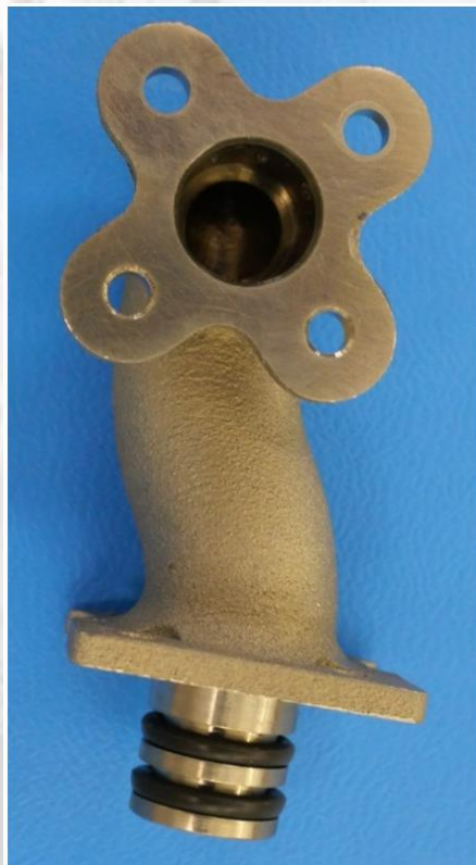
Presumed rust spots on secondary pump manifold.
