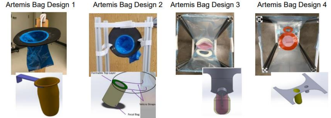
Evaluation #1 - Artemis Bag low-fidelity prototypes (4 designs)
