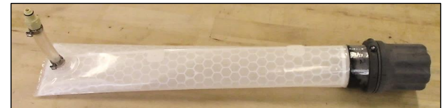
High-fidelity prototype of the Collapsible Contingency Urinal (CCU) hardware (with male interface)
