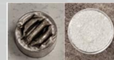
Pleated (L) Sintered (R) Filter
