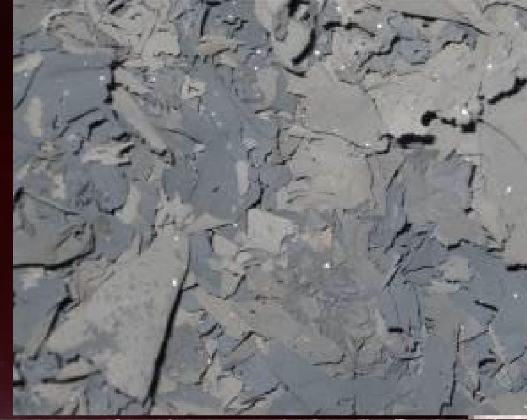
Carbon formed in pH Matter CFR. Credit: Z. Greenwood, et al. 2018.
