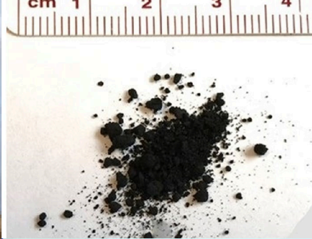
Bosch carbon from rotary kiln CFR. Credit: B. C. Stewart, et al. 2022.
