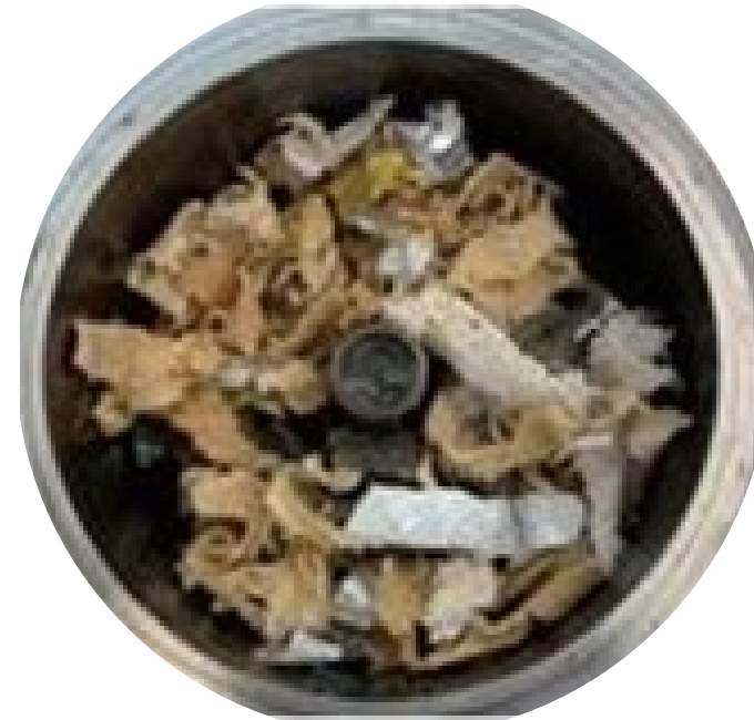
OSCAR Reactor with ~22grams of shredded TCPS tiles
