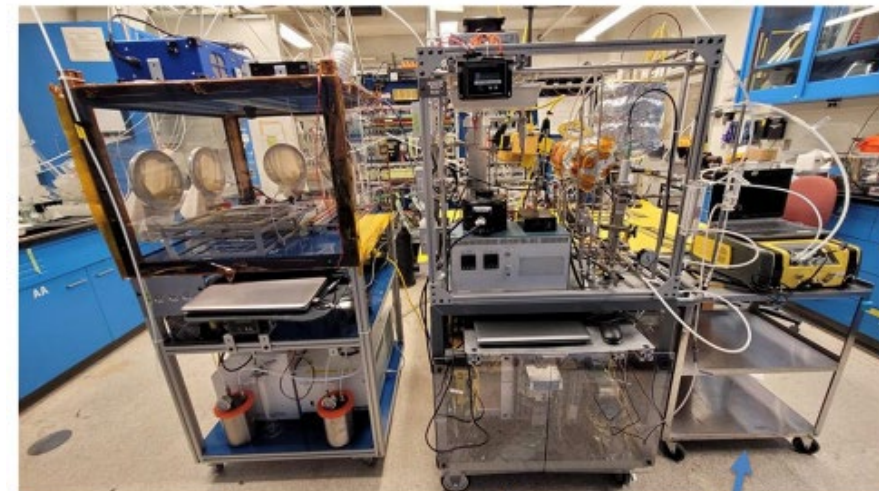
TCPS loaded with trash for testing (at ARC)
