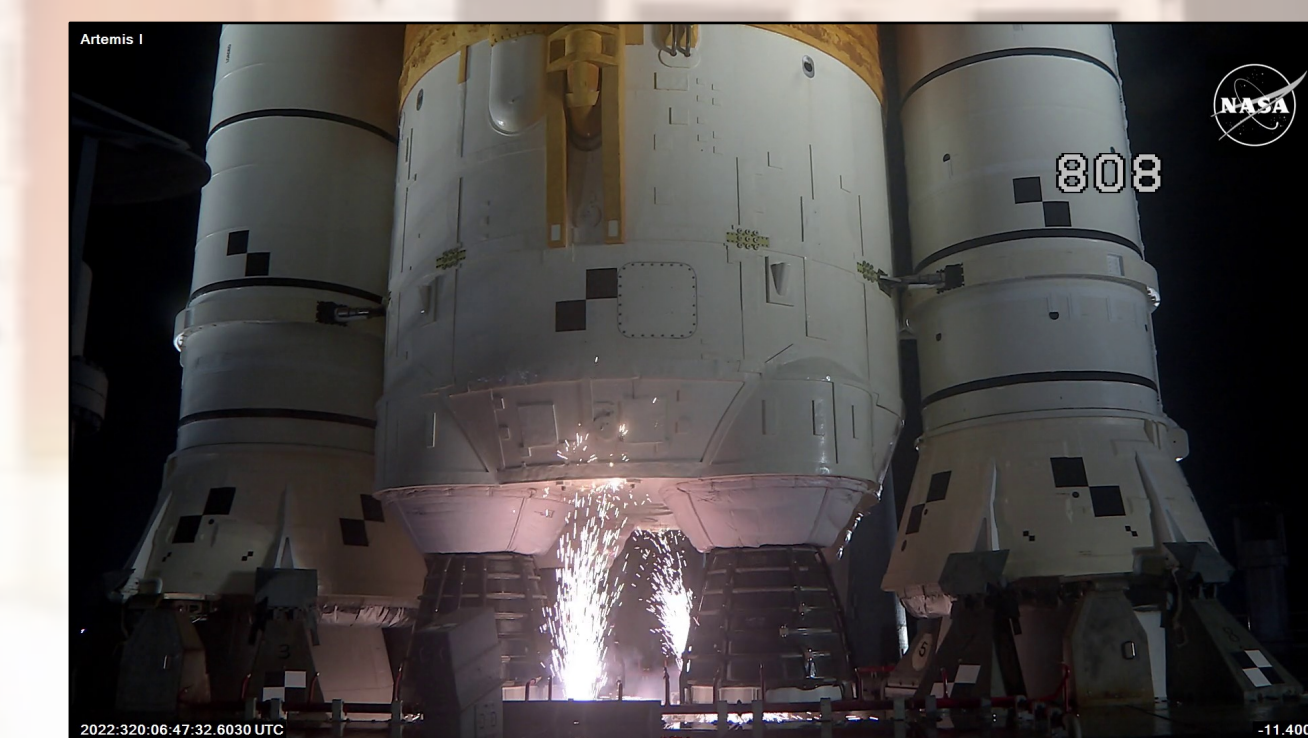
Hydrogen Burn-Off Igniters during SLS Hold-Down
