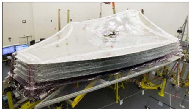
Figure 21. Sunshield deployment test.
