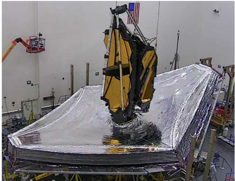
Figure 22. Final deployment test of the JWST observatory.
