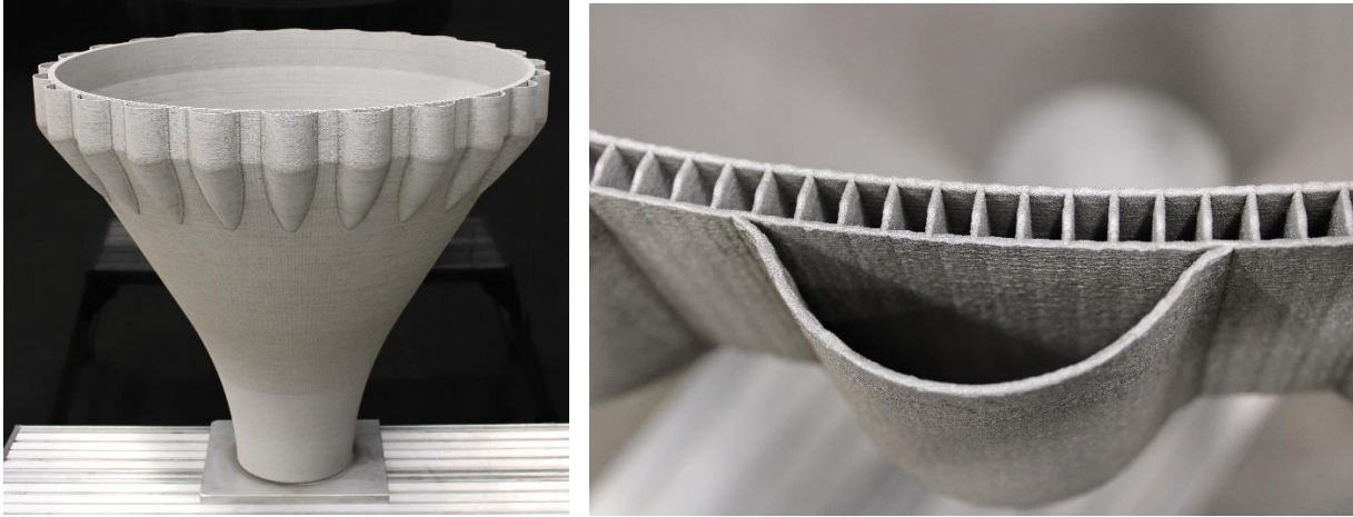
Figure 3. Demonstrative Large-Scale Regeneratively Cooled Nozzle.
