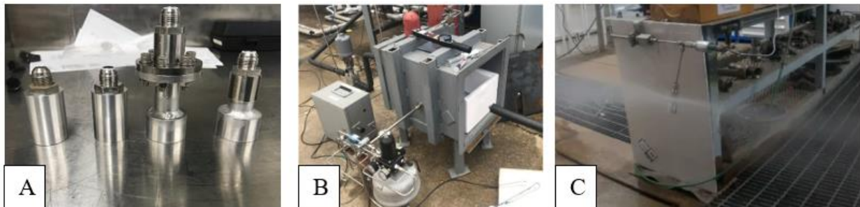
Figure 5. Port Testing Overview. (A) Four Test Fixtures Tested, (B) Testing Setup, (C) Burst Testing of the Port Samples.
