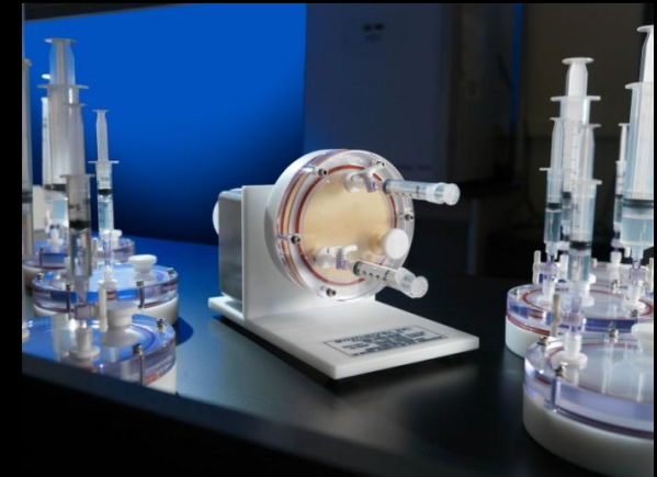
Low fluid shear culture conditions in the RWV prompted the term Low Shear Modeled Microgravity (LSMMG) environment
