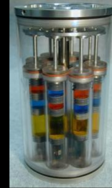
Fluid Processing Apparatus (FPA), an example of in-flight hardware
