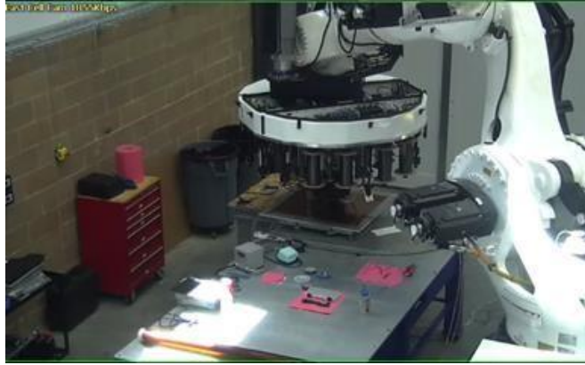
Figure 5. Electroimpact® VSS-HP laser-assisted thermoplastic AFP Developmental Head.
