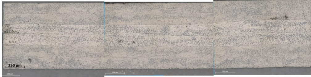
Figure 15. Photo-microscopy of PEEK Panel-6 from first ICAT processing experiments.
