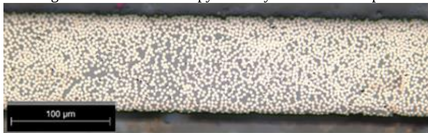
Figure 9. Photo-microscopy of Victrex AE250/IM7 slit-tape.
