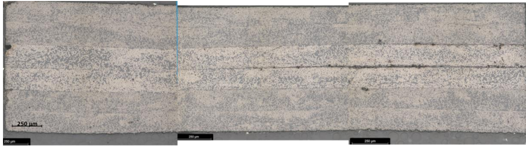
Figure 16. Photo-microscopy of PEEK Panel-1 from first ICAT processing experiments.
