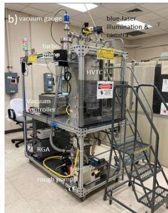
Thermal High Vacuum Chamber (THVC) test stand designed and built in-house at MSFC
