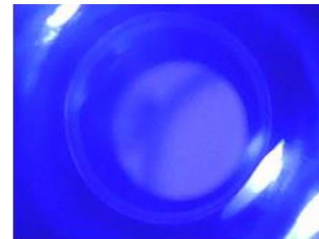
Image of the melt taken by the camera mounted on the top of the HVTC under blue-laser illumination at 1,400 C.
