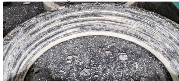
Figure 5. DPA Photo of the Sleeve Contamination.
