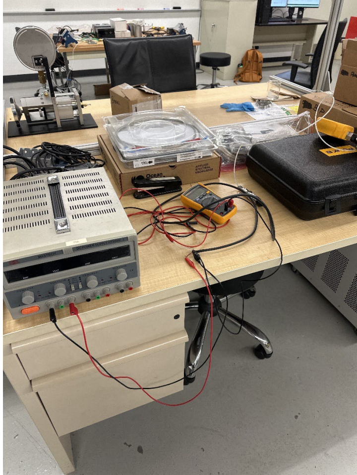
Preliminary Pressure Transducer Testing Setup
