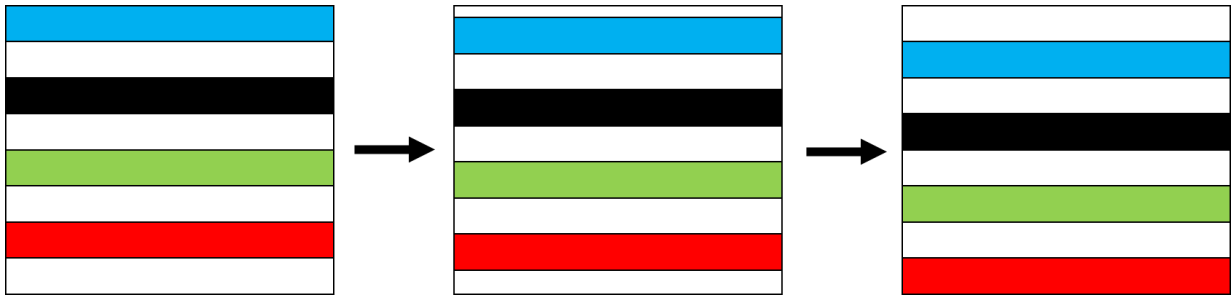
Fig. 7. A pictographic representation of the test image used during irradiation. The color bars slowly scroll across the screen and will wrap around the sides of the screen.
