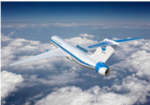
Figure 1.—STARC-ABL aircraft concept in flight. (Credit: NASA)
