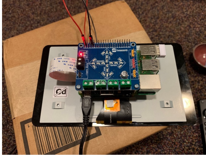
Figure 4: Initial electronics setup using SB Components motor controller.
