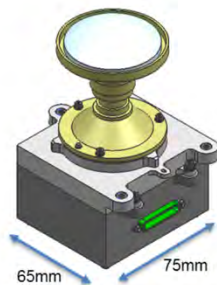
Figure 5.18.3: Diagram of Mars 2020 EECAM Camera [AFSS-11]
