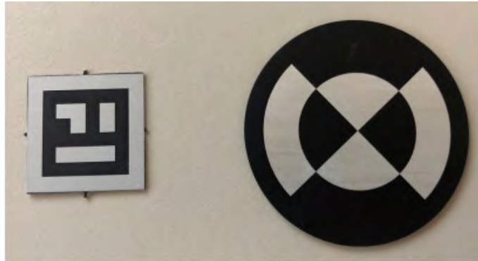
Figure 5.18.7 Left: Standard April tag Right: Mars Science Laboratory marker [AFSS-39]
