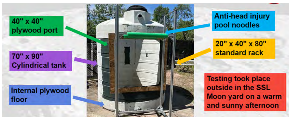
Figure 6.16.3: X-HAB Testing Setup
