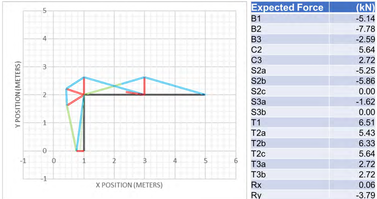
Figure 7.7.1: Extended configuration plot and expected forces
