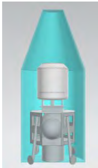
Figure 6.13.2: PLM and Lander Within Falcon Heavy Fairing Envelope
