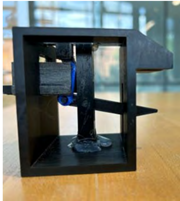
Figure 5.6.2: Latching mechanism 3D print
