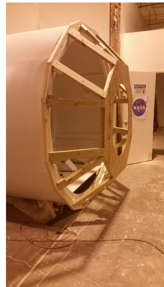
Fabricated end cap and installed window
