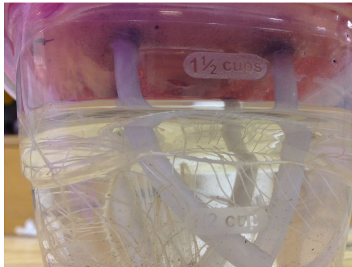
Figure 20: Roots growing into the water reservoir and some noticeable debris.
