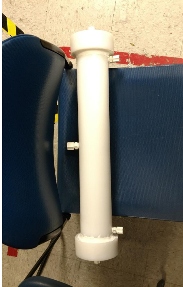
Figure 69. ILS assembly without compression assembly.
