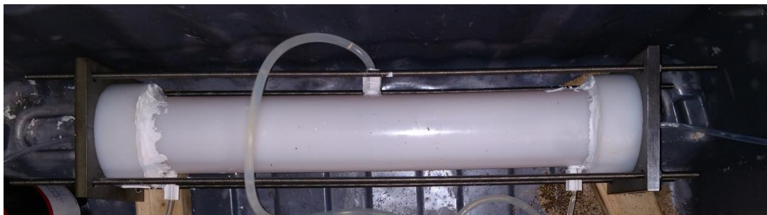
Figure 70. ILS contactor with compression assembly installed.
