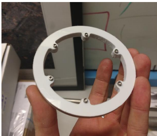
Figure 23. Screw Lock Ring with screws.
