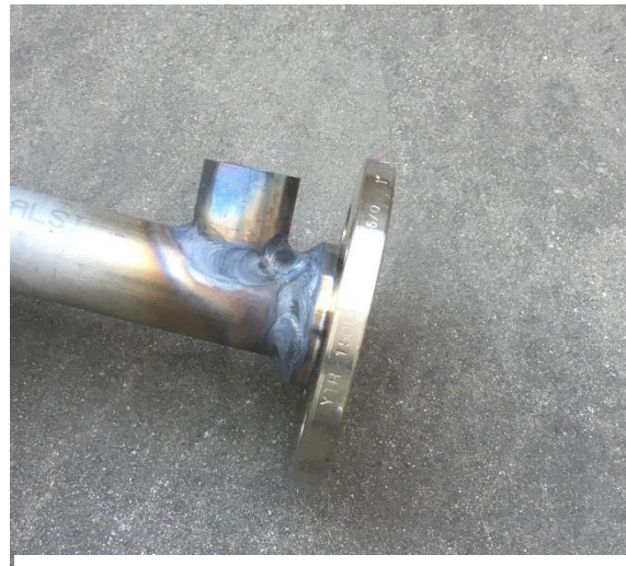
Figure 50. One end of WCS outer pipe assembly.
