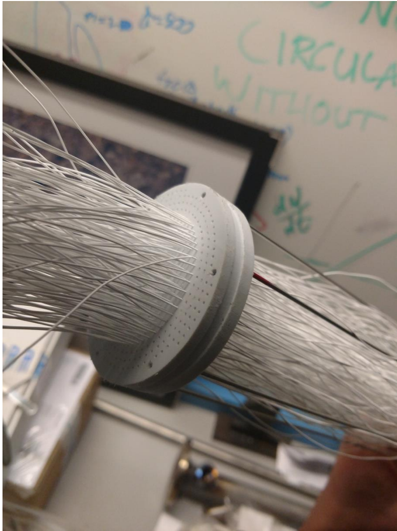
Figure 63. Threading fibers through the fiber guides.
