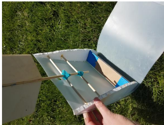
Figure 26. Completed drop box for low gravity testing
