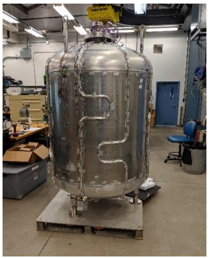
CryoFILL Tank Uninsulated on a Support Stand
