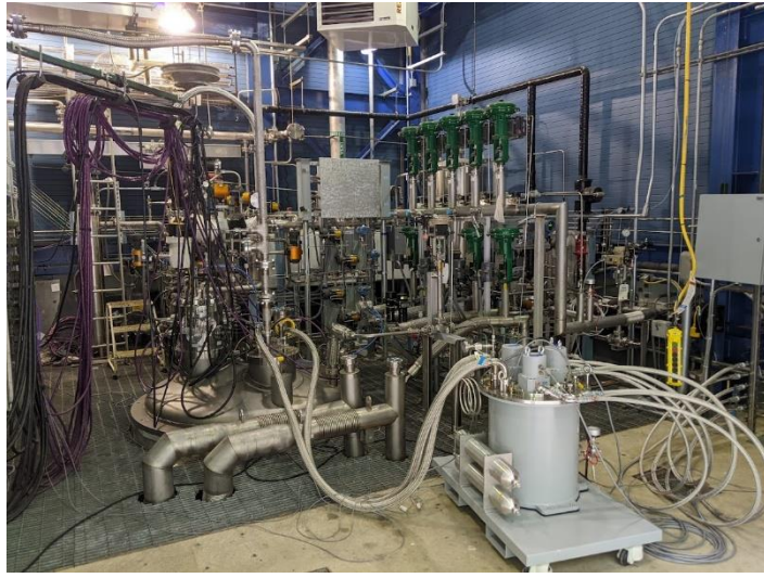
NASA GRC SMiRF Facility with Prototype Test Article in Vacuum Chamber. Industrial cryocooler coldbox in the foreground.
