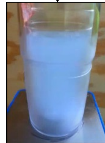
Appx. 255g of liquid MOX being stirred
