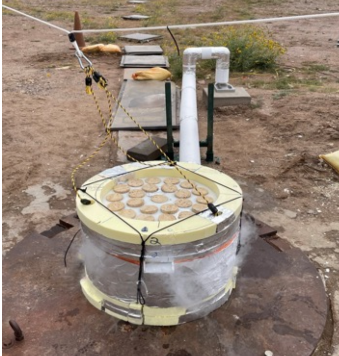
LMA PRC Pathfinder Test Article (30 Kg of propellant)
