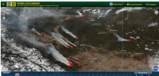
Figure 2: FIRMS US/Canada Fire Map displaying active fire detections observed on May 05, 2023 over Alberta, Canada. The active fire detections are derived from the VIIRS instrument onboard NOAA-20. The active fire detections are displayed on a VIIRS NOAA-20 Corrected Reflectance true color composite imagery showing dense smoke emanating from the active fires.
