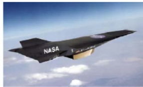
X-43A Scramjet with supersonic Combustion ramjet engine
