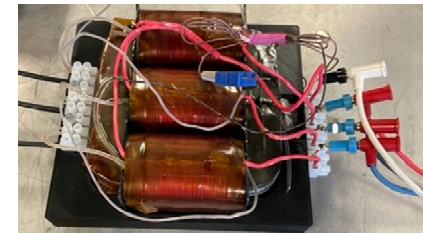
3.3 kVA single-phase design (3x for 10 kW)
