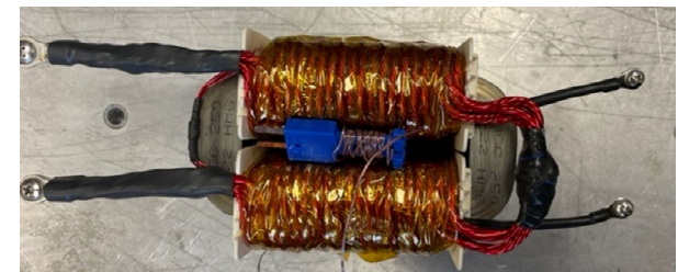
3.3 kVA single-phase design (3x for 10 kW)
