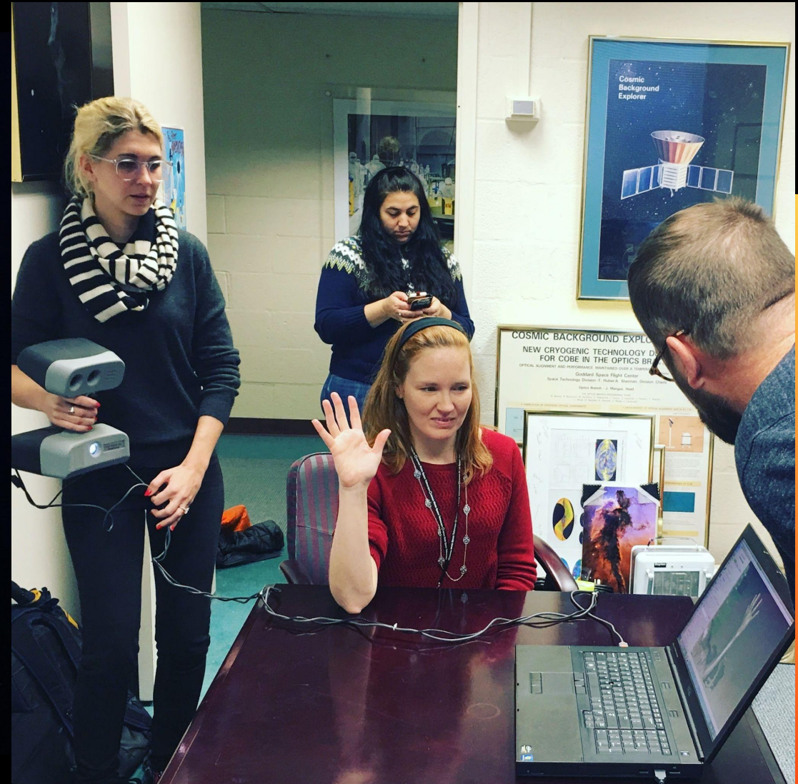
Scanning the arm of Dr. Amber Straughn for “Exploration” using an Artec Eva structured-light 3D scanner. (Image by Ashley Zelinskie)
