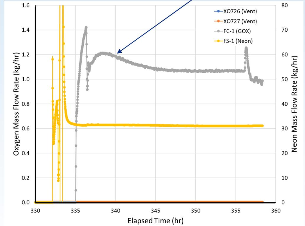
Cryocooler is running at a constant fan speed for each test and the gas input/liquefaction rate is allowed to float to maintain tank pressure
