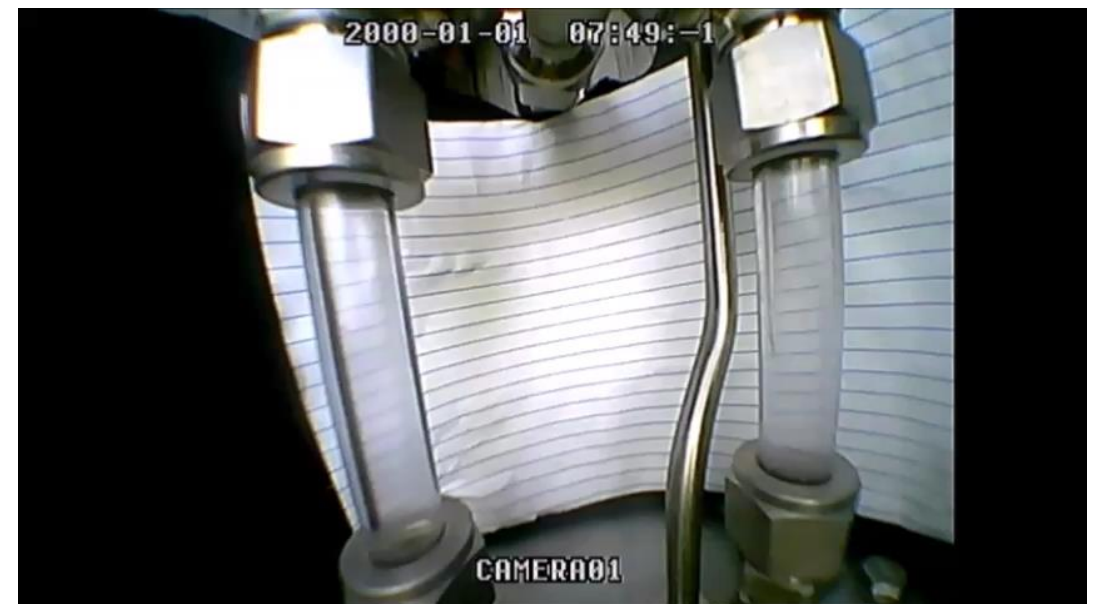
Video footage showing liquid slosh after the transition into microgravity (left) and video confirmation of breakdown during flow testing in microgravity (right).
