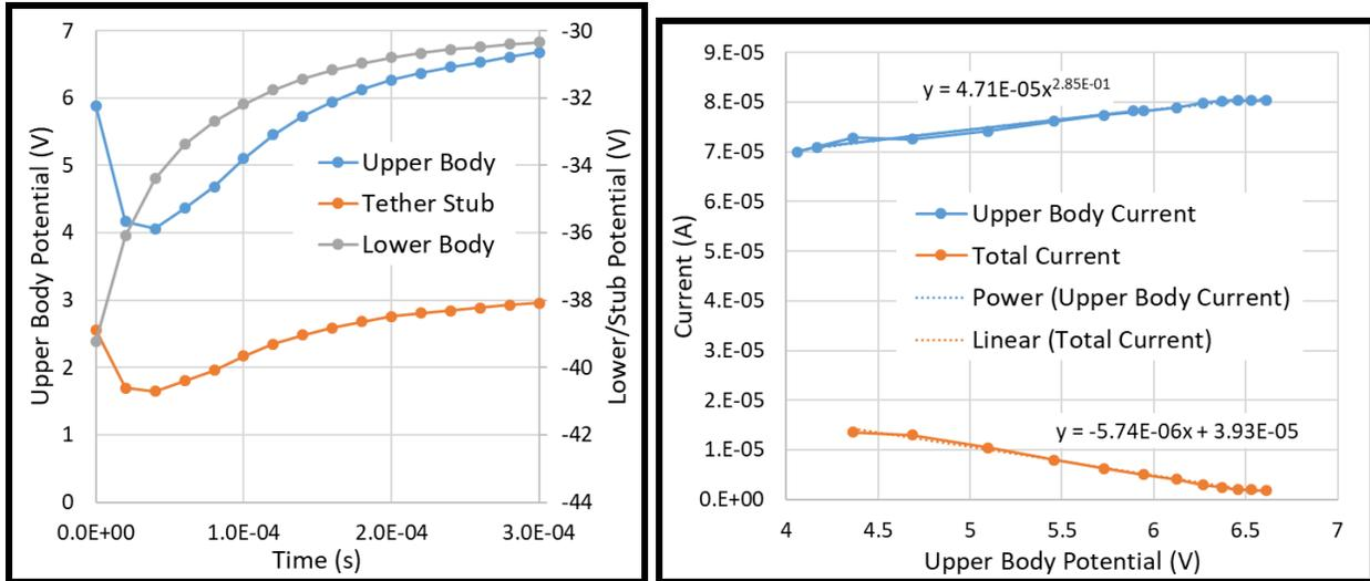
Figure 24. For the resistive (100 kΩ) case, potentials of the three components versus time (left panel), and upper body and total currents versus upper body potential (right panel).
