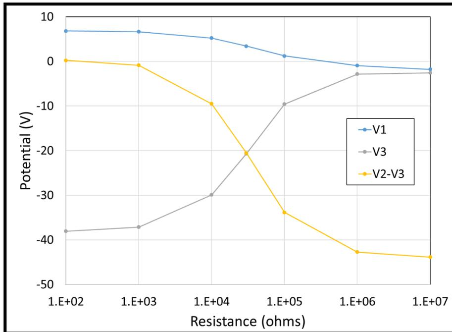
Figure 14. Potential of upper body (V1, upper curve), lower body (V3, upward sloping curve) and the measurable difference (V2-V3) as a function of tether root coupling resistance. Note that the end points (100  $\Omega$ , 10 M $\Omega$ ) are actually the shorted (Section 3.3) and floating (Section 3.4) cases respectively.
