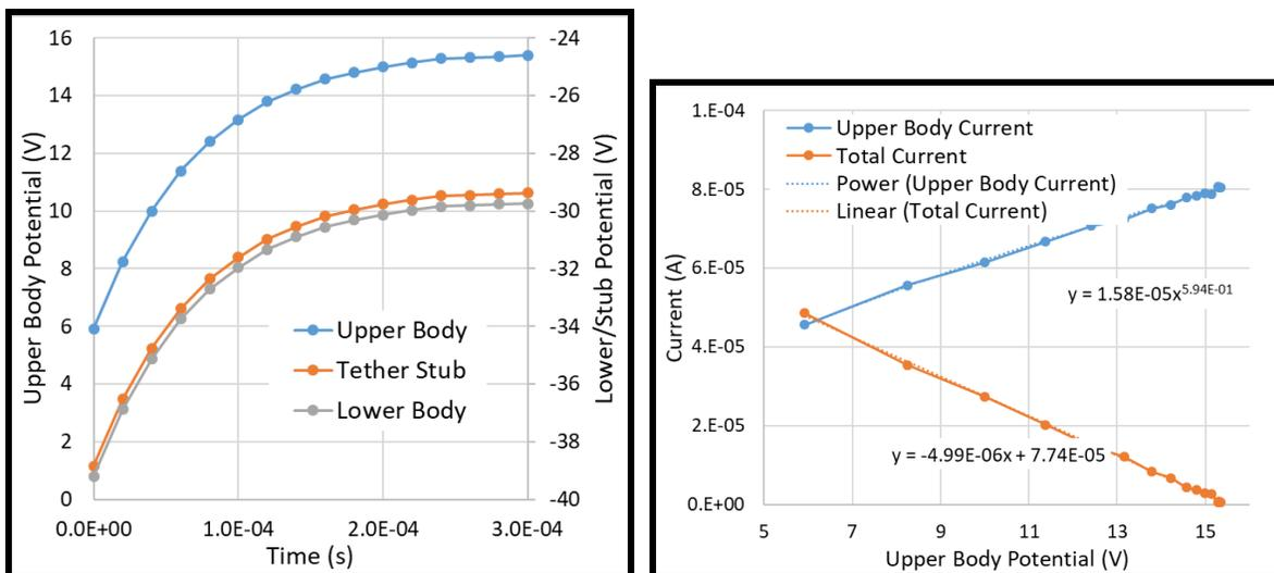
Figure 26. For the case of smaller upper body, individual body potentials vs. time (left panel), and upper body and total currents vs. upper body potential (right panel).
