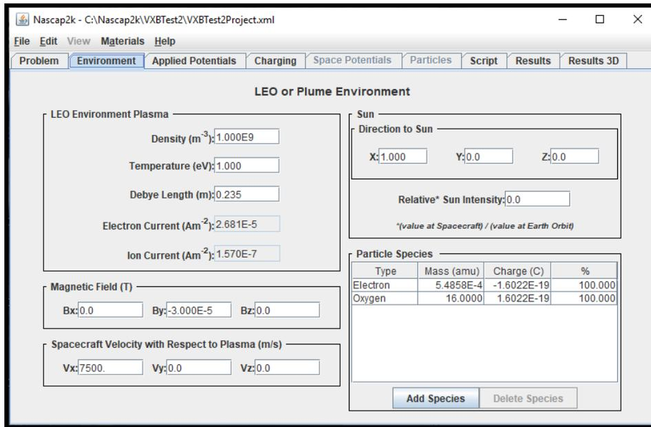
Figure 11. Environment tab values for the Tether example.
