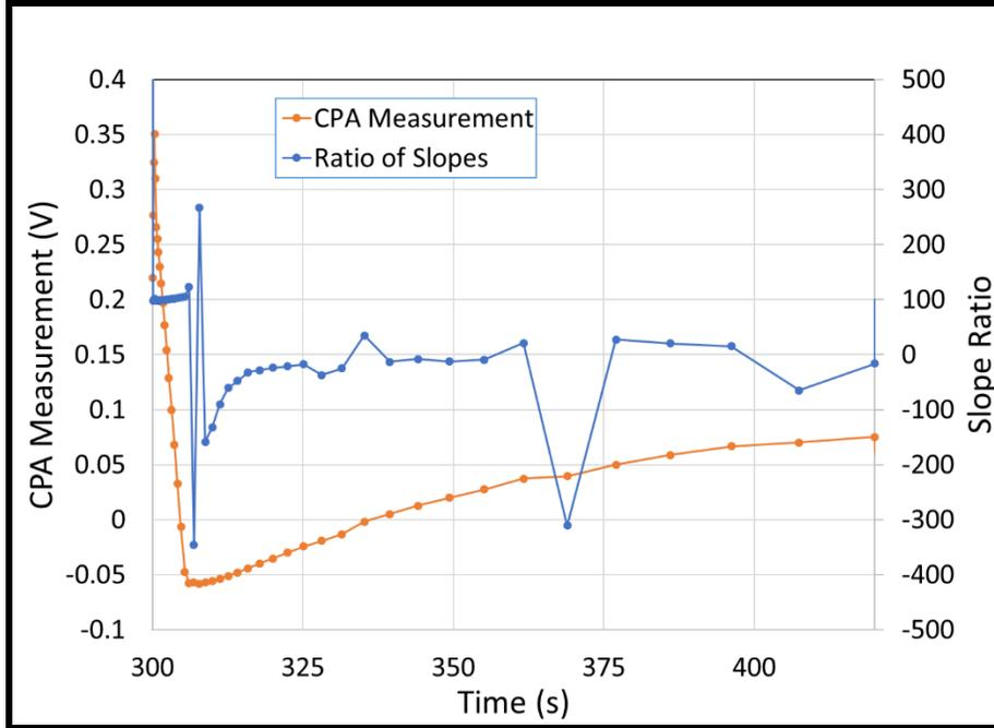
Figure 9. Time dependence during the sunlit period of the CPA measurement voltage (left axis), and the ratio of the time derivative of the surface differential potential to the time derivative of the CPA measurement (right axis).
