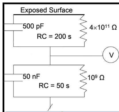
Figure 1. Simplified circuit for the Charge Plate Analyzer. The upper portion of the figure represents the properties of a dielectric coating, while the lower portion of the figure shows the measurement circuit.
