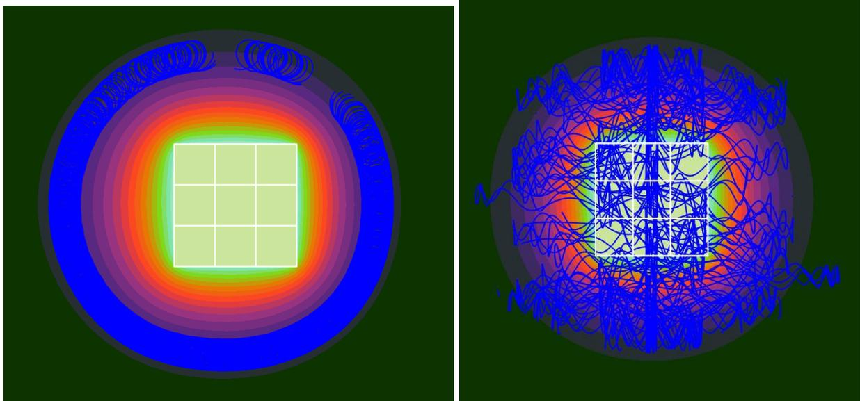
Figure 21. Particle trajectories of electron macroparticles generated along  $Y=0$  contour (left panel) and along  $X=0$  contour (right panel).
