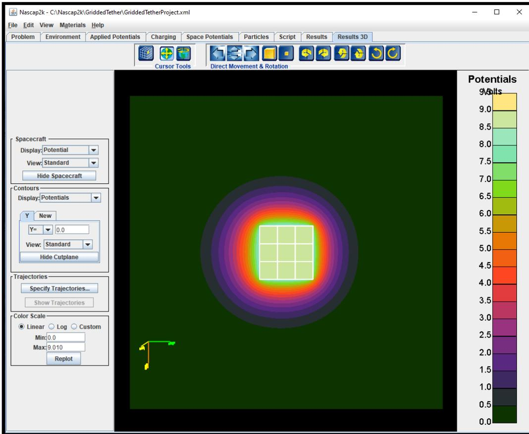
Figure 19. Potential contours around the upper body.
