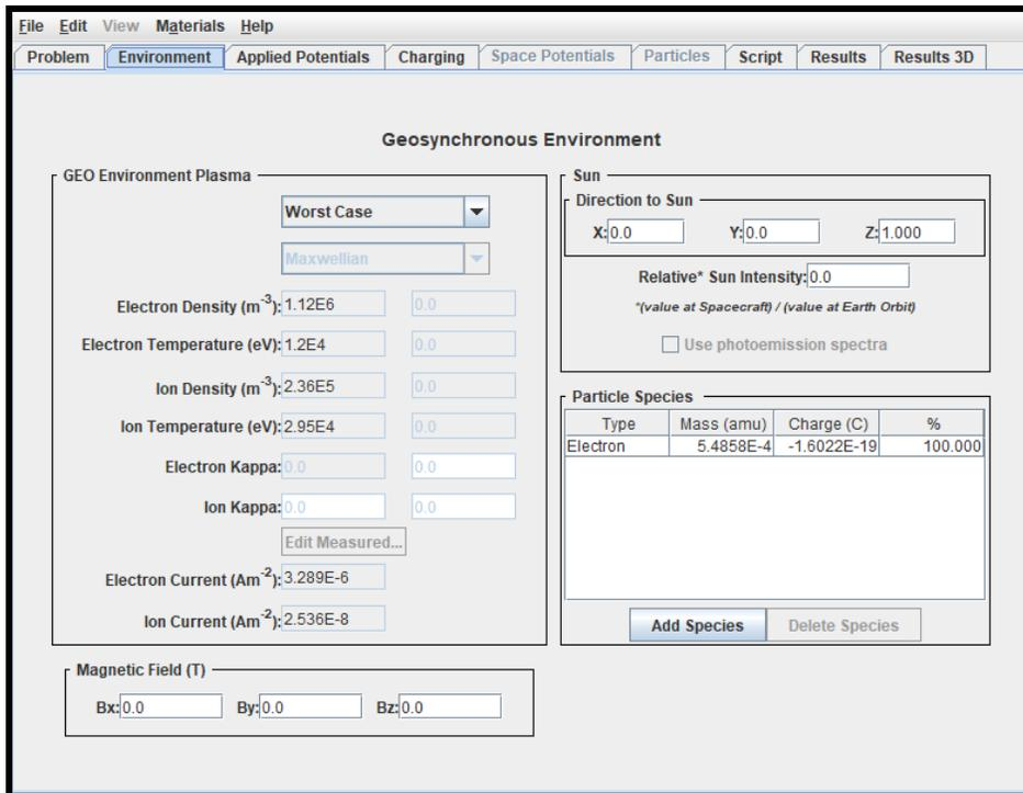
Figure 3. Environment tab values for the CPA example.
