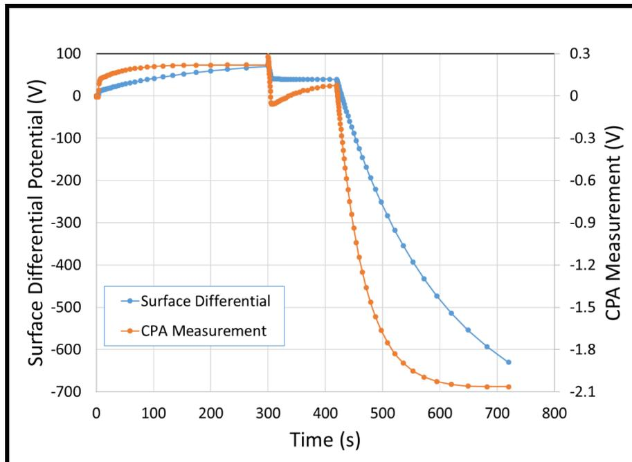
Figure 7. Time history of CPA surface differential potential (left axis) and measurement potential (right axis) for the eclipse, sunlit, and shadowed portions of the calculation.
