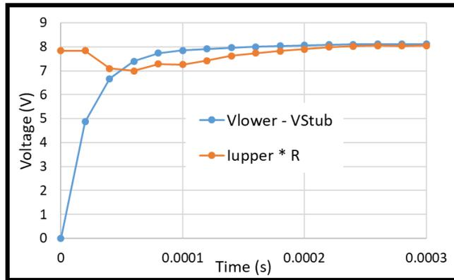
Figure 25. Measured lower body to stub potential difference (blue curve), compared with value inferred from upper body current flowing through 100 kΩ resistor (orange curve).
