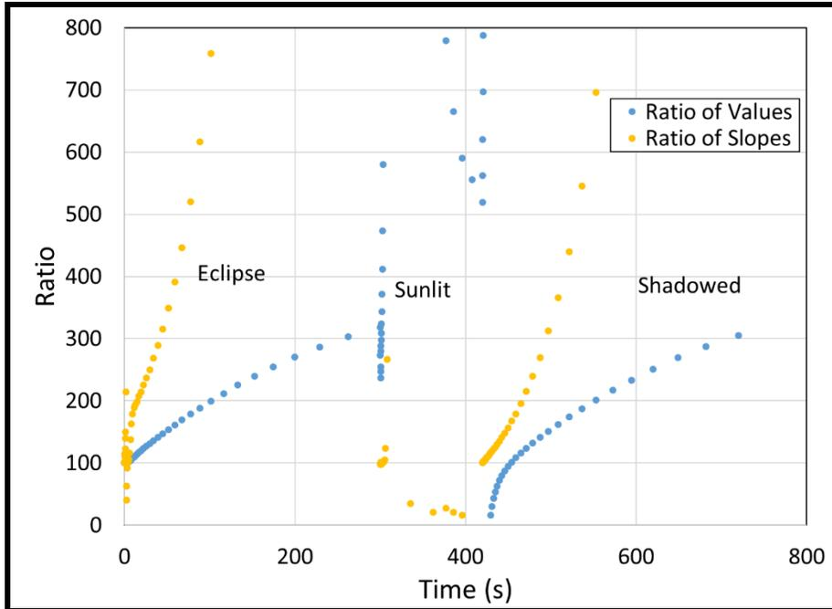
Figure 8. Time dependence of the ratio of the surface differential to the CPA measurement voltage, and the ratio of the time derivatives of those quantities.
