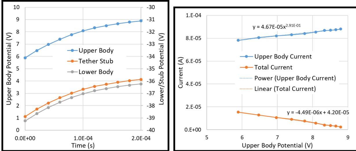
Figure 18. Left Panel: Time behavior of the upper (left axis) and lower body (right axis) potentials. Right Panel: Potential dependence of the upper body current (which is negative) and the total current for the shorted case.
