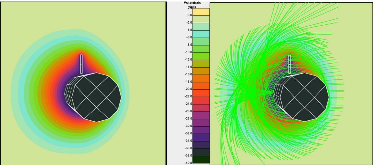
Figure 22. Sheath potentials (left panel) and ion trajectories (right panel) near the lower body.
