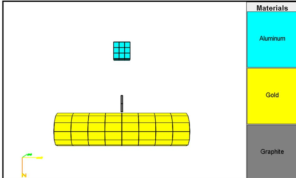
Figure 10. View of tether example object prior to moving upper body to -200 m. (View from  $-X$  direction with  $Z$  downward.)
