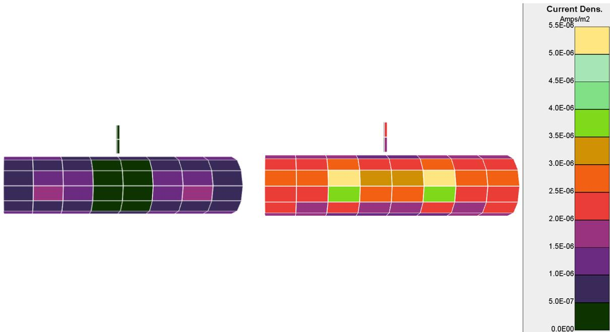
Figure 23. Incident ion current density on wake side (left), and ram side (right) of the lower body.
