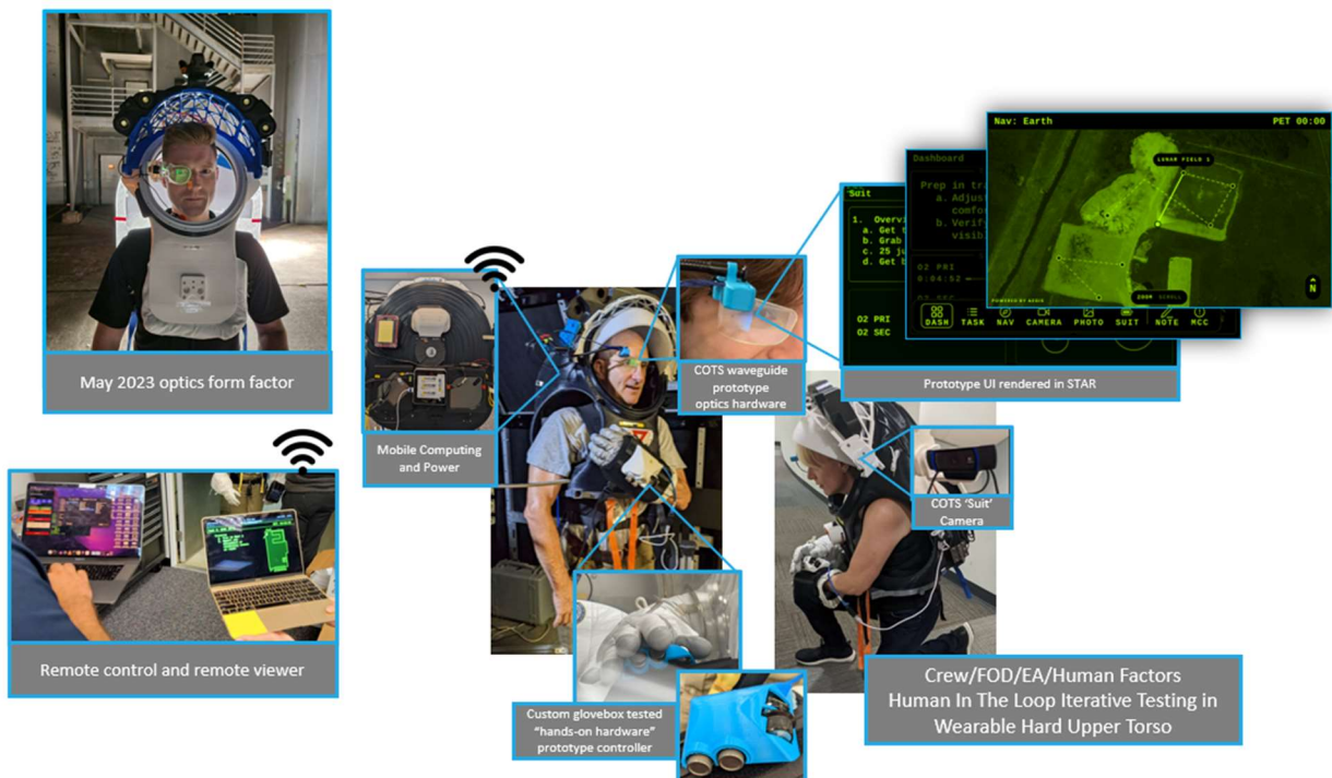
Figure 2. The Joint AR system end-to-end components as tested via Joint AR avionics architect Tyler Garrett, and crewmembers Don Pettit and Kate Rubins (left to right)
