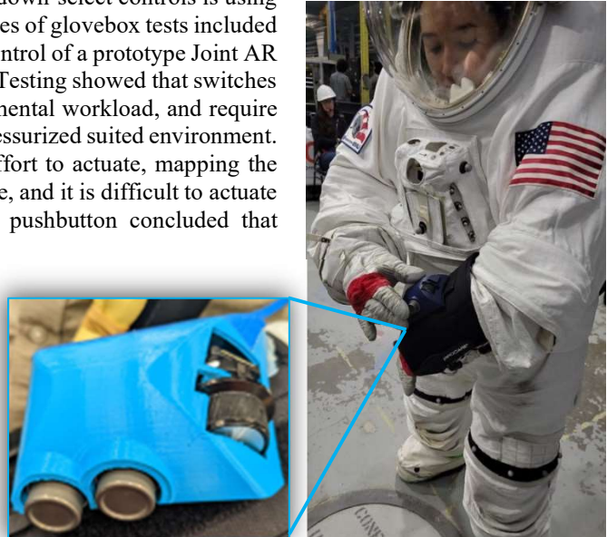
Figure 1. Design of the Joint AR physical hand controller represented on an xEMU pressurized suit fit check during ARGOS testing
