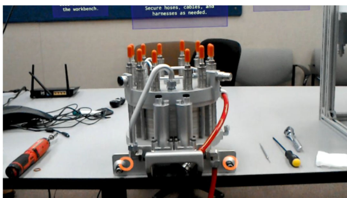
Figure 9. Augmented reality view while installing OGA cell stack on a workbench to perform repair/replacement of a pressure transducer
