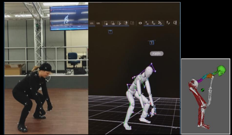
OptiTrack Motion Capture use with Digital Astronaut and Microgravity Exercise Device Analysis Projects
